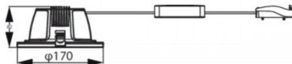
Cut-out hole diameter - Ø150mm
