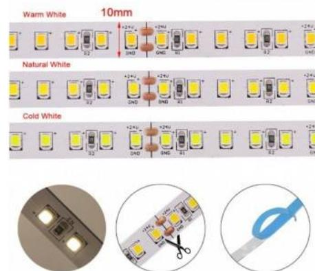
**Tira LED 24V-DC - 9W/m - monocolor - 10mm - IP20 - Rollo 50 metros - 60 chips/m - Corte c/10 cm**
