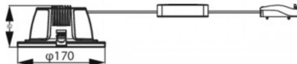
Cut-out hole diameter - Ø150mm
